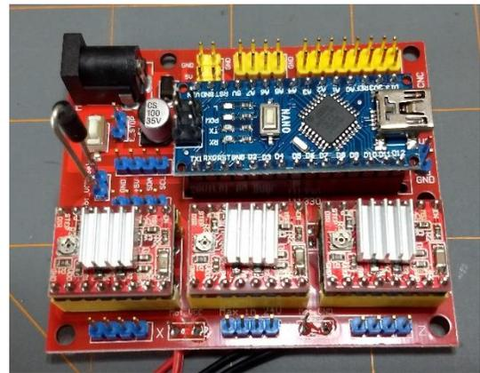
Figure 4-13 A4489 Motor Boards Installed
