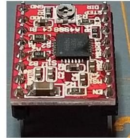
Figure 4-14 A4489 Motor Board Before Heat Sink is Installed
