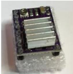
Figure 4-16 DRV8825 with heat sink installed
