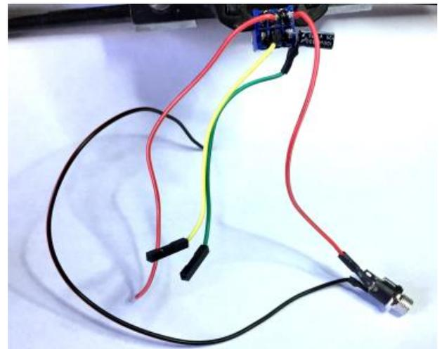
Figure 4-9 Completed power harness
