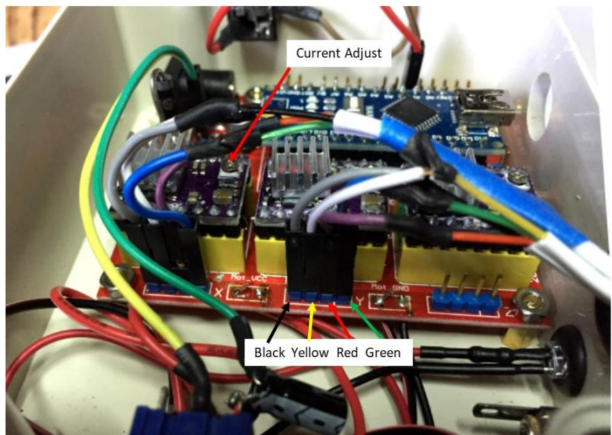
Figure 4-28 DEC Stepper Driver Connections, RA motor is similar to the DEC motor connections shown
