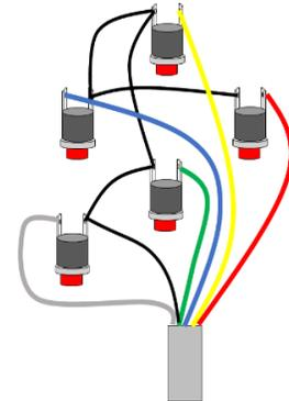
Figure 8-1 Keypad Wiring Diagram
