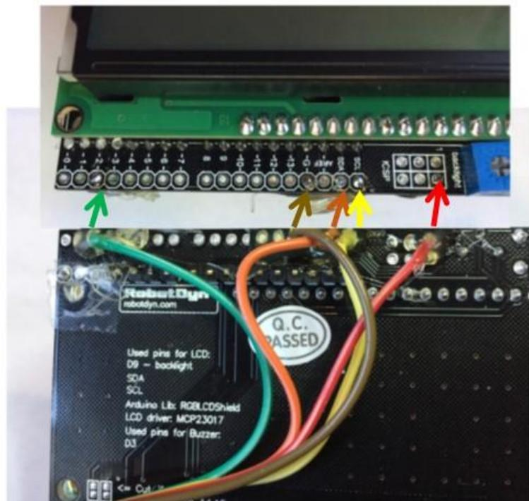
Figure 4-30 RGB LCD Connections
