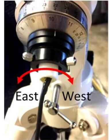
Figure 4-20 Tilt switch in housing on back of RA shaft.
