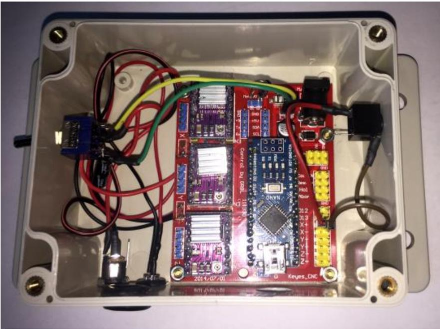
Figure 4-23 Enclosure with tilt switch jack installed
