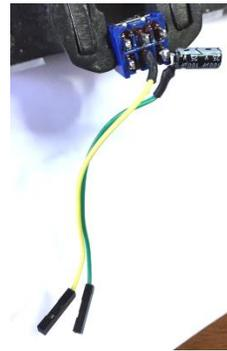
Figure 4-6 Reset Circuit
