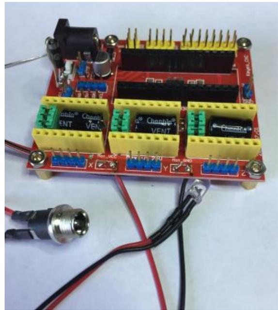
Figure 4-10 Control board power connections
