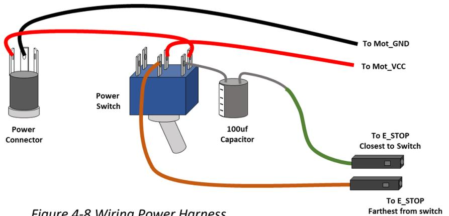
Figure 4-8 Wiring Power Harness
