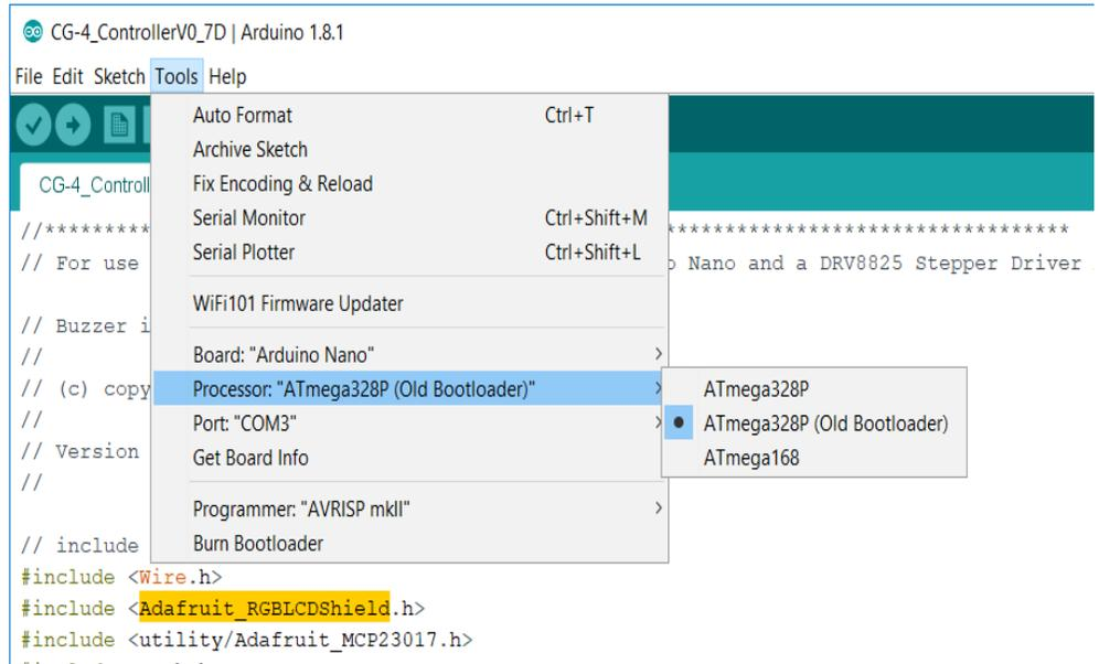
Figure 3-1 Set Processor/Bootloader
