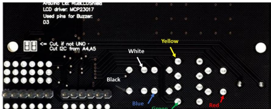
Figure 8-3 Where to solder the Keypad wires on the back of the LCD Display
