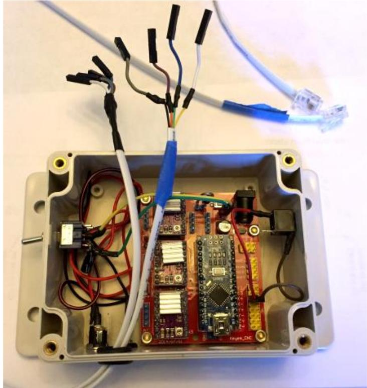
Figure 4-27 Stepper cables
