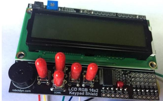
Figure 4-29 RGB LCD Display with button extensions
