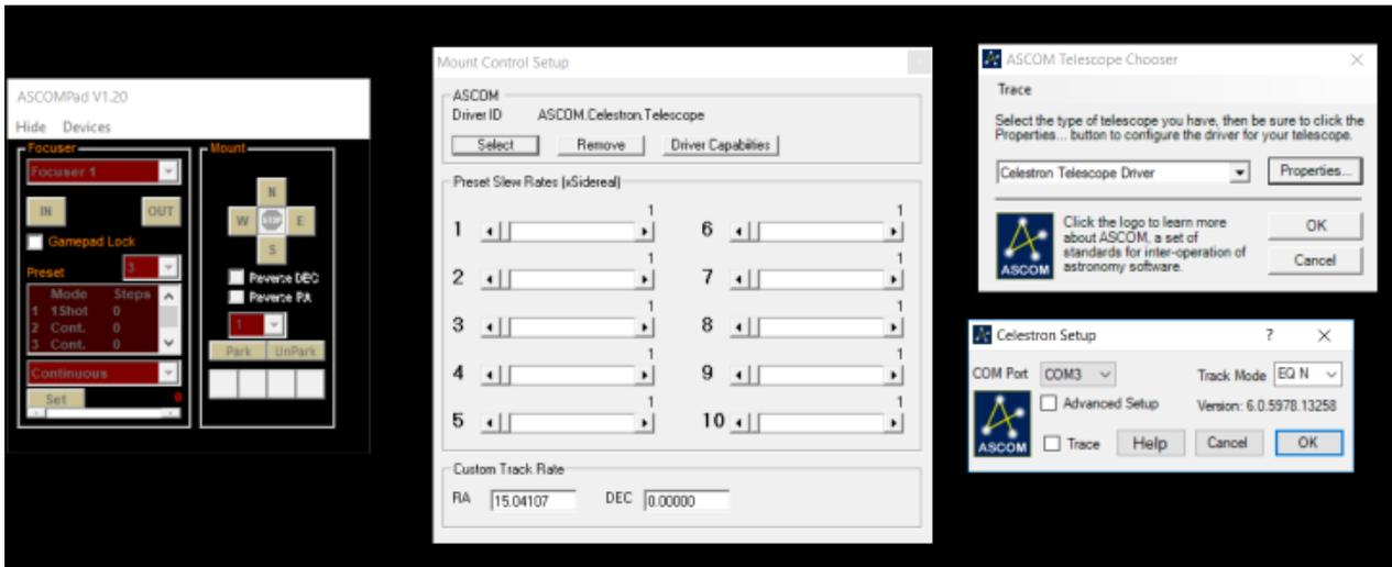
Figure 6-2 ASCOM PAD Setup Windows
