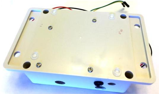
Figure 4-18 Bottom of Enclosure with screws and feet installed
