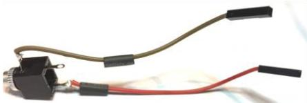
Figure 4-22 Tilt switch jack with wires attached
