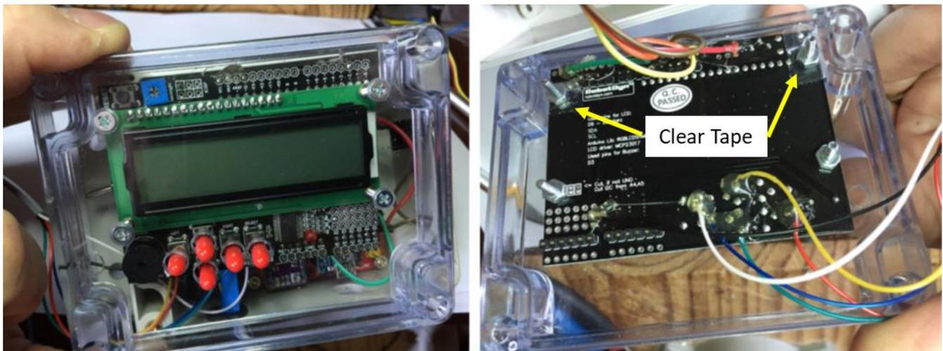
Figure 4-32 Display mounted in clear top.
