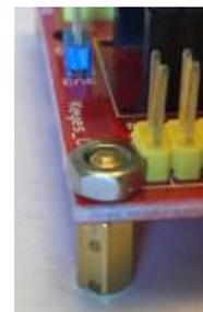
Figure 4-17 Attach Stand Offs to Control Board
