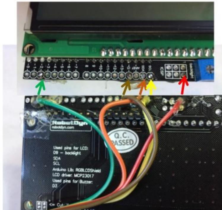
Figure 4-30 RGB LCD Connections
