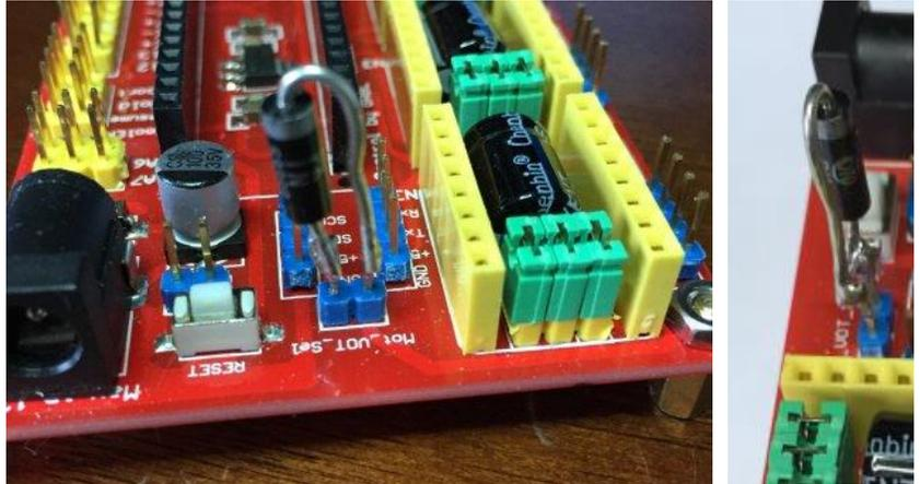
Figure 4-4 Solder Zener Diode across jumper pins.
