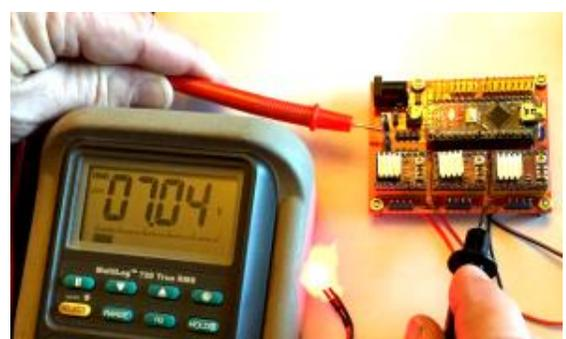
Figure 4-12 Voltage with Nano installed
