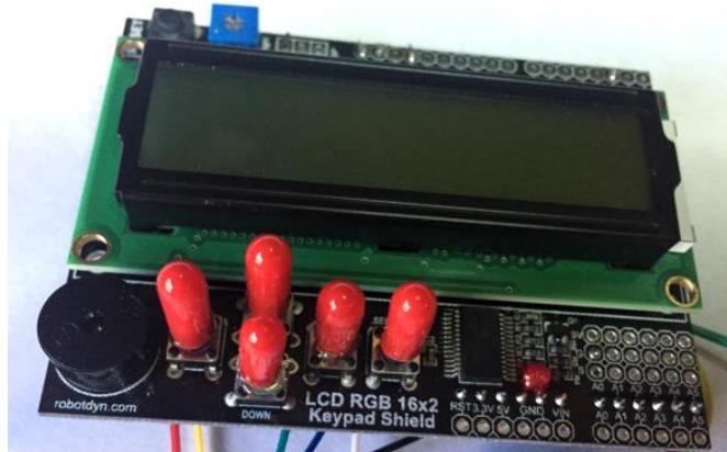
Figure 4-29 RGB LCD Display with button extensions
