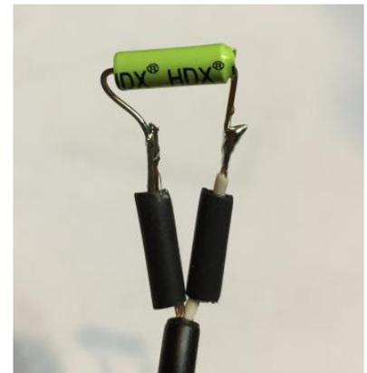
Figure 4-21 Tilt switch attached to phono cable
