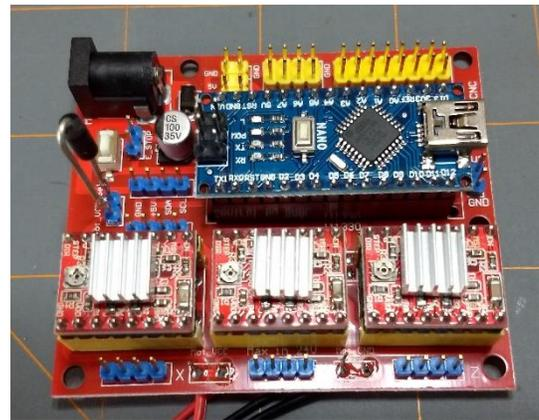
Figure 4-13 A4489 Motor Boards Installed
