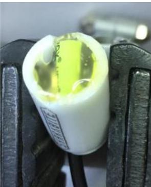
Figure 4-26 Tilt Switch glued into cap
