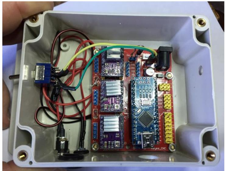
Figure 4-19 Power Harness Installed
