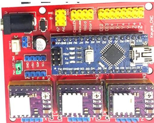
Figure 4-15 DRV8825 motor boards installed
