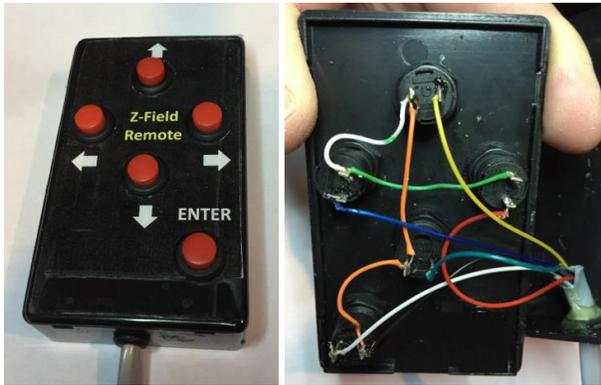
Figure 8-2 Remote Keypad outside and inside
