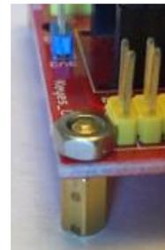
Figure 4-17 Attach Stand Offs to Control Board
